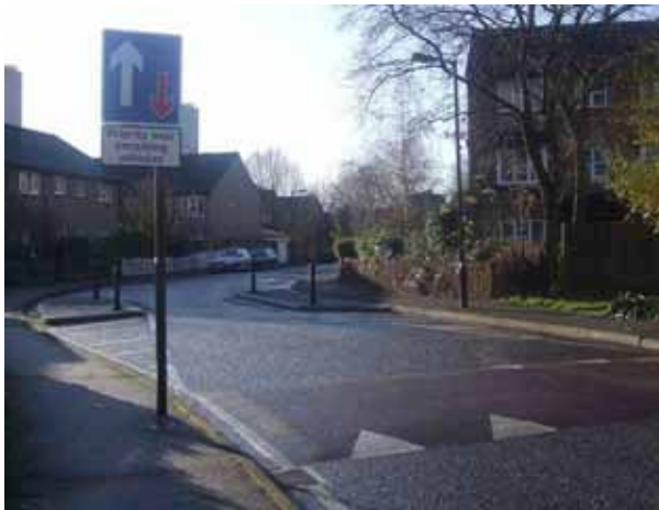
Figure 4.7 Pinch-point with priority operation
